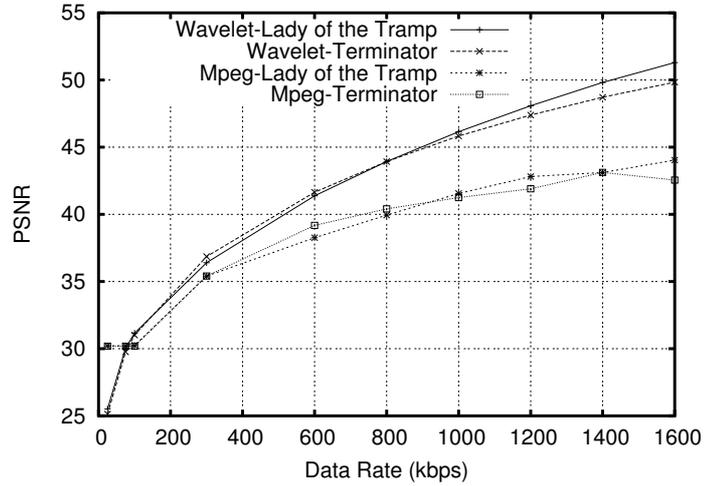
Fig. 4. Average video quality as function of encoding target bit rate for wavelet 3D-EZBC and MPEG-4 encoded movies.
