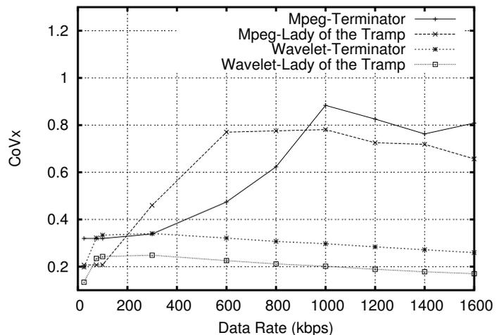
Fig. 1. Coefficient of variation as function of target bit rate for wavelet 3D-EZBC and MPEG-4 encodings.
