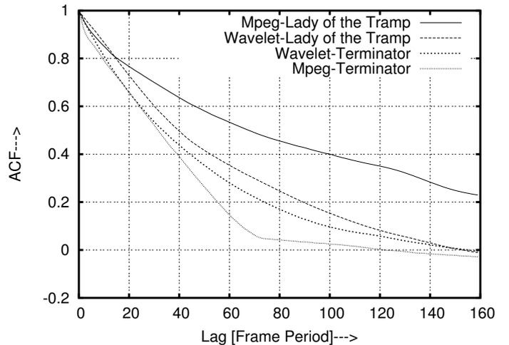
Fig. 3. Autocorrelation as function of lag  $k$  for wavelet 3D-EZBC and MPEG-4 encodings.
