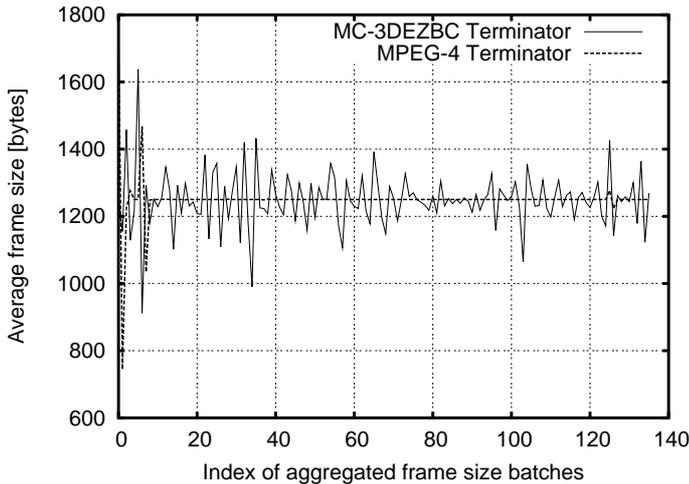
Fig. 2. Aggregated frame size trace ( $a = 792$ ) with target bit rate 300kbps for *The Terminator* encodings.
