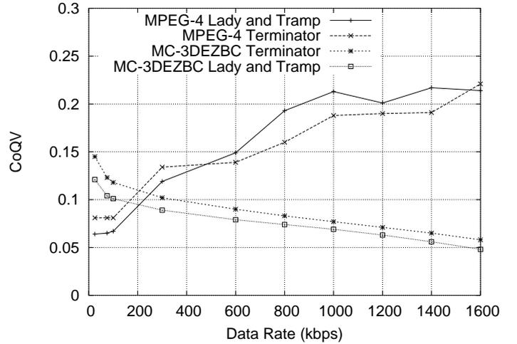
Fig. 5. Coefficient of quality variation for wavelet 3D-EZBC and MPEG-4 encoded movies.
